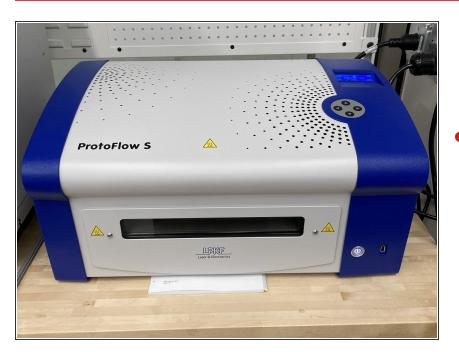
The ProtoFlow is a reflow oven that follows specific temperature curves to melt solder paste and cure solder mask/silkscreen.
