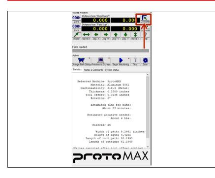
After importing the part reset the home position of the nozzle by clicking the button indicated in the picture
