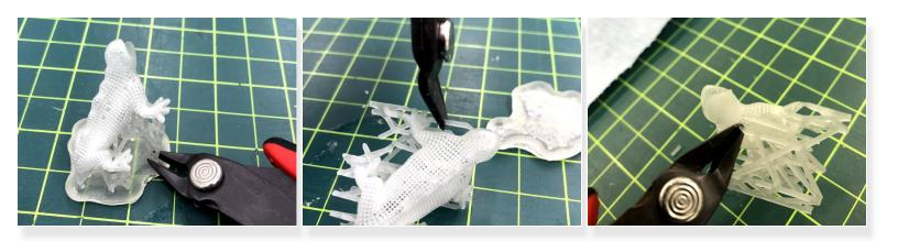
• Bring the cured parts to the mechanical space to remove supports
