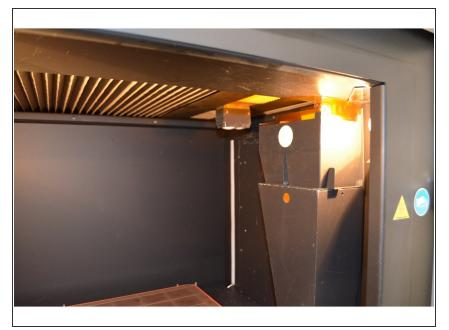
Reinstall all the components of the tip cleaning assembly, as well as the debris chute hood
