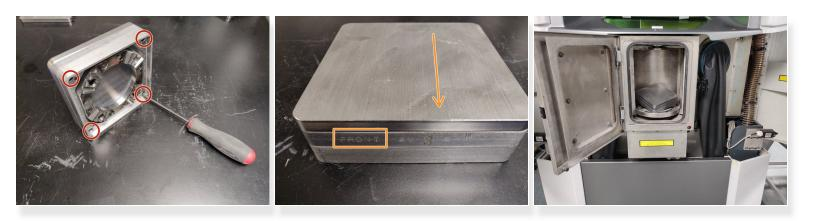
• Attach the build plate to the base plate using (4) 4mm screws
