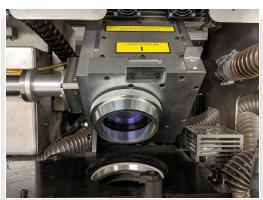
• Pull the plunger out from the left side and lift the box by the tab on the right
