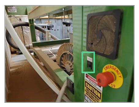
Shutdown the computer, after a successful computer shutdown, flip the on/off EZ router switch.
