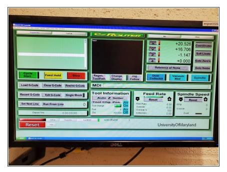
To load G-Code, simply find the file on the removable drive, and drag it over the MACH software, and release it.
