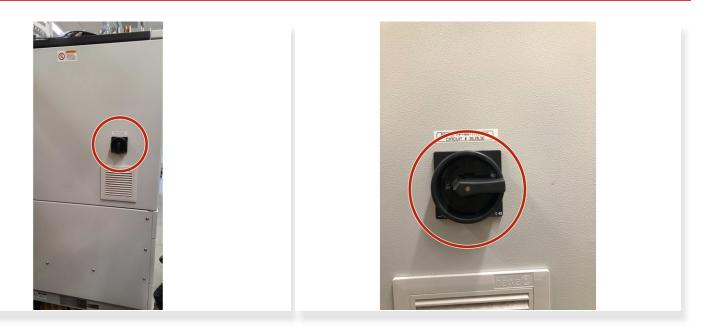
Flip the switch on the back of the machine from on to off.
