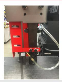
Ensure that the right red guard is secured back to the machine and that the blade is behind it. The
