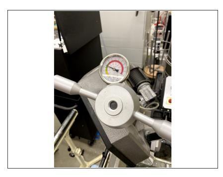
On the horizontal bandsaw, you want to make sure the blade is within the green on the blade tension gauge.
