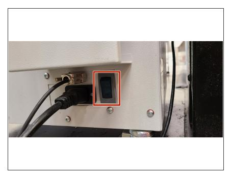
Switch the vacuum cleaner off before opening the machine. The power switch is highlighted in the red box.
