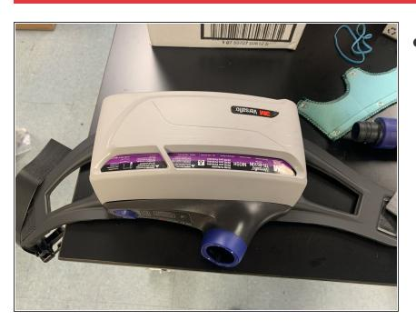
Place the light grey cover on top of the filter with the cut out towards the top (closest to hose hole) until you hear a click and all the sides are flush with the waistband.
