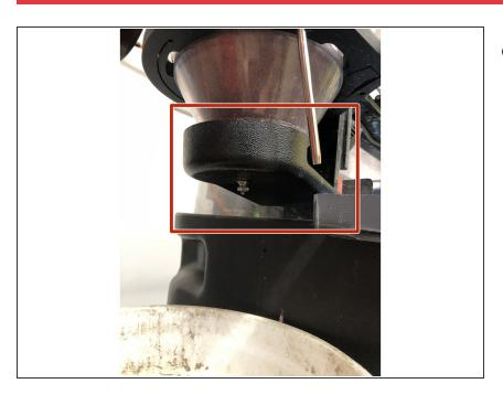
Put splash guard back on along with the washer and splash guard nut.
