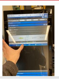
Now, finally, you can see the tool in your magazine and you can tell the software to measure the tool length in the screen as shown and you will be all set!
