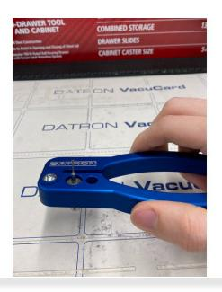
After removing the old tool, simply slip the new tool in the collet whilst still holding on the clamp.
