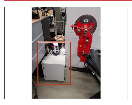
The Datron has an external vacuum that sits behind the machine next to the lathe.
