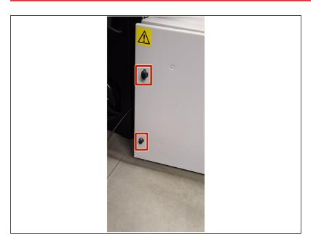
Twist both knobs to open the door. It should pop open when it has been properly unlocked.
