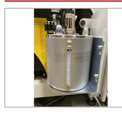
Check the canister down to the bottom left and make sure that the clear tube has liquid in it, preferably more than a quarter up from the bottom at least.
