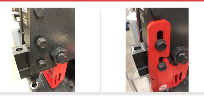
Use the 3/4in socket to remove and replace the bolts
