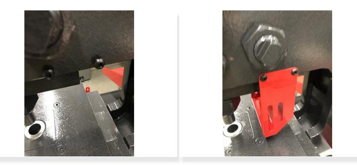
• Use the 9/64th T handle to remove the screws and then tighten the guard back into place.
