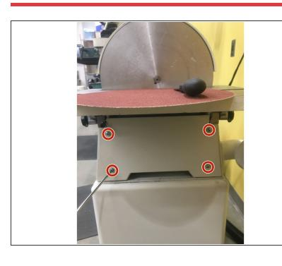
Using a screwdriver, unscrew the four screws holding in the lower cover. Once the cover is removed, vacuum up any dust.
