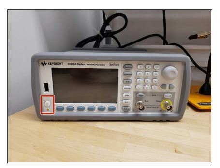
The power button is located on the front of the machine in the bottom left corner.
