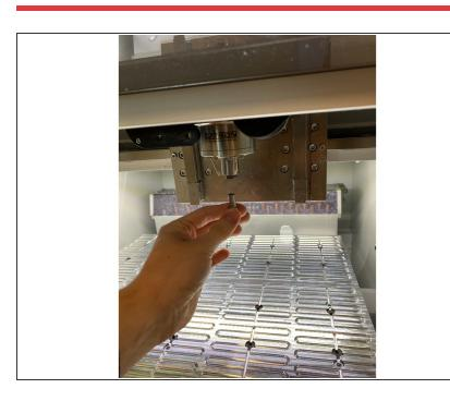
You can now remove the tool, and if you wanted to do a tool not from the spindle, you simply just pull it out of the magazine.
