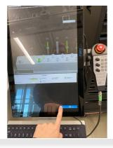
Now insert the tool into the magazine, pushing it down firmly, then selecting okay on the screen saying the tool has been changed.
