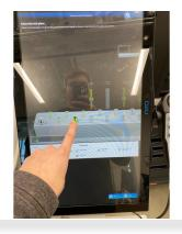
Once back in the screen under tool management, select the correct tool you are replacing the previous tool with from the warehouse and select the location you want it to take in the tool magazine.
