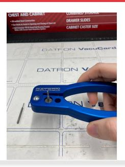
After selecting your new tool to insert, place the collet in the shown device and clamp down a little bit, just enough to release the tool.
