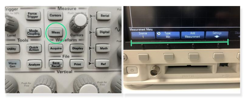
• To measure different properties of your displayed signals, you can press the "Meas" button in the Measure section of buttons. This will display a set of options for adding measurements on-screen.
