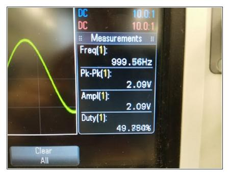
Measurements appear constantly on screen in the lower right corner, and update in real time.
