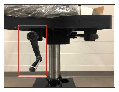
Once desired height is reached, tighten the left bolt to lock the table height in place.
