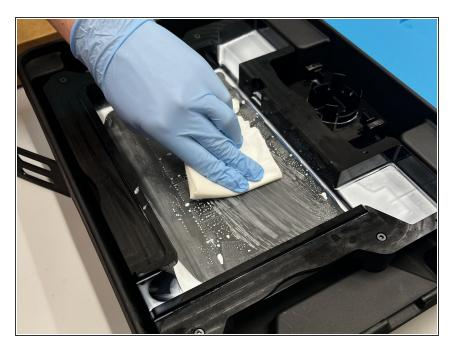
⚠ Gloves must be worn at all times when handling uncured resin or cleaning the tank or other tools.
