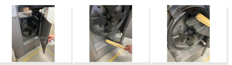
Open the door and using a brush, sweep the dust and shavings to the opening on the right. Be sure to dust off the wheel and door as well.
