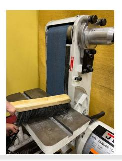
• Use a brush to clean off the dust on the tables where the disc and the belt are
